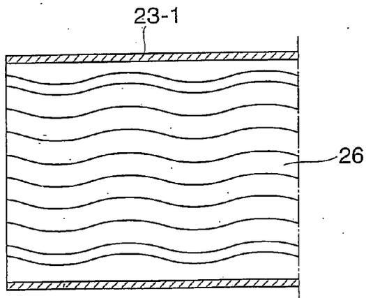
**FIN STRUCTURE, HEAT-TRANSFER TUBE
