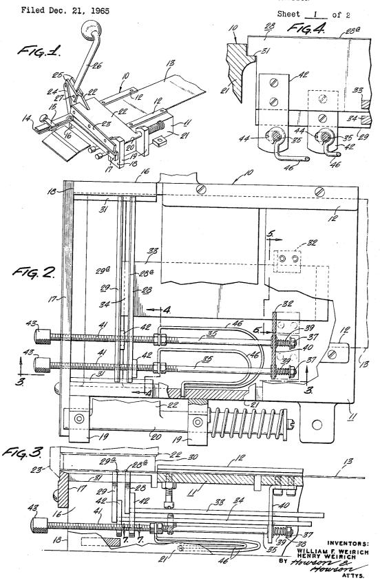
DEVICE FOR CREASING AND CUTTING SLOT INSULATION
