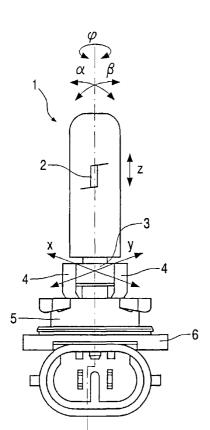
(57) Abstract: A lamp cap with a spring cup for retaining a lamp burner (1), for which it is proposed that the spring cup has at least three spring legs (4) which each have substantially only one degree of freedom. The spring legs (4) are arranged such that the three degrees of freedom enable a displacement possibility of the spring cup in a displacement plane and are linearly independently aligned in this displacement plane.
