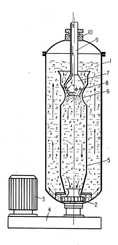
DEVICE FOR ADMIXING A GASEOUS AND A LIQUID PHASE
