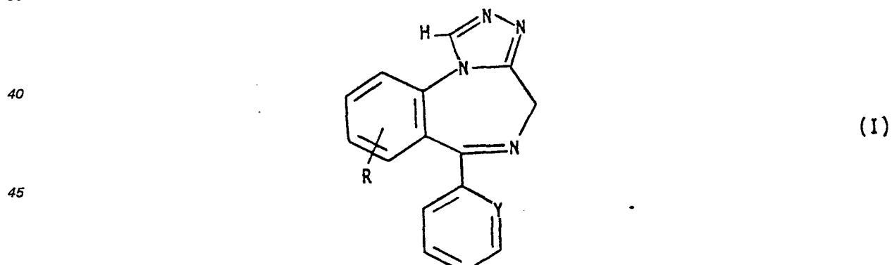
50 in an inert liquid solvent, under essentially neutral pH conditions for up to 5 hours, at a temperature sufficient to dissolve the formula I compound and to crack the paraformaldehyde to a reactive form of formaldehyde. R is H, F, Cl, Br, CF<sub>3</sub> or NO<sub>2</sub> and Y is N, CH, CF or CCl. The starting material may be estazolam.
