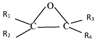
where at least one of said R<sub>1</sub> – R<sub>4</sub> is selected from a two to fifteen carbon (C2 – C15) acyclic group, a C2 – C15 aliphatic group and a C2 – C15 ethers. An epoxide according to Formula 5 1 is sometimes referred to herein for convenience as **ADM1**.
