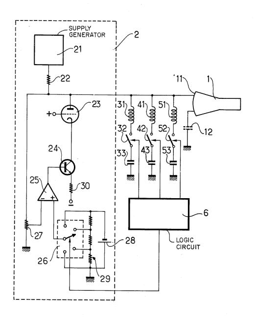
HIGH VOLTAGE RAPID SWITCHING CIRCUIT
