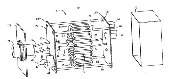
(57) Abstract: A filter package includes a pair of spaced circuit boards; a magnetic core between the circuit boards; a plurality of windings on the core extending to at least one of the boards; and a plurality of conductor bars mechanically fastening and electrically interconnecting the circuit boards.
