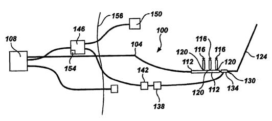
(57) Abstract: An air bubble detection system includes an air bubble detector which is disposed downstream from a syringe or manifold used during an angiography procedure. The air bubble detection system monitors contrast medium being injected into the patient and creates an alarm or other indication if the air bubble exceeds any desired threshold.
