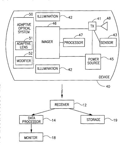
(57) Abstract: Device, system and method for adaptive imaging and adaptive in-vivo imaging. For example, an in-vivo imaging device (40) may include a lens (51) and a modifier (52) to modify a physical property or an optical property of said lens.
