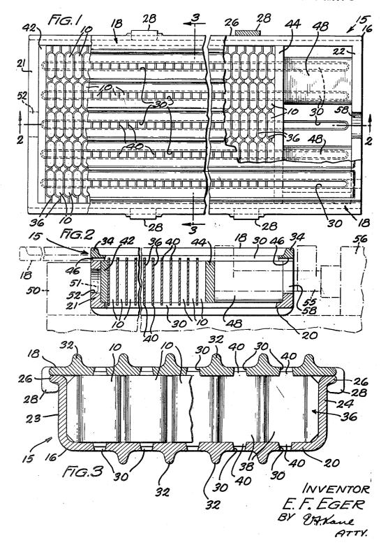
FIXTURE FOR USE IN COATING PARTS OF ARTICLES
