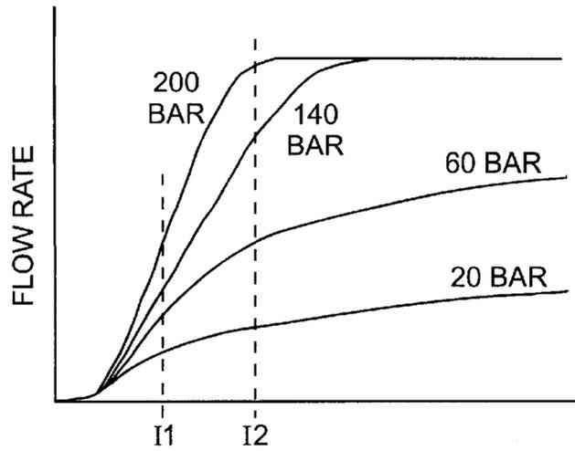
FIG. 1 ACTUATOR CURRENT
