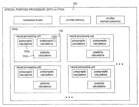
(57) Abstract: A special purpose processor (SPP) can use a Field Programmable Gate Array (FPGA) or similar programmable device to model a large number of neural elements. The FPGAs can have multiple cores doing presynaptic, postsynaptic, and plasticity calculations in parallel. Each core can implement multiple neural elements of the neural model.
