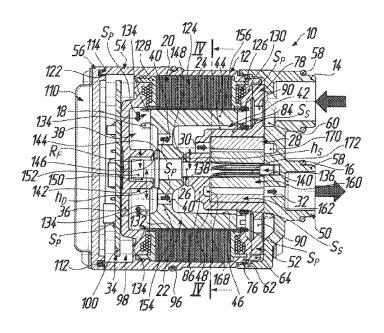
in part via the annular gap and undergoes a deflection at the partition wall, cooling the latter before it passes through the rotor passage to the suction inlet.
