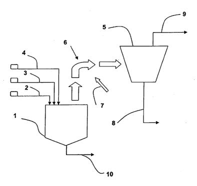
(57) Abstract: A method of operating mechanical separation devices at high temperatures to separate various volatile metals, metal halides and metal oxides to produce high purity materials, in particular to recover zinc or zinc oxide from electric are furnace dust.
