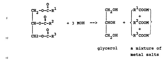
The above reaction is indicative of 100% saponification of the starting triglyceride. However, less than 100% saponification can occur which when overbased to a "Newtonian" system (D) gives a useful product.
