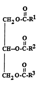
wherein R<sup>1</sup>, R<sup>2</sup> and R<sup>3</sup> are each independently saturated or unsaturated aliphatic hydrocarbyl groups containing from about 8 to about 24 carbon atoms, wherein the vegetable oil comprises soybean oil, rapeseed oil, sunflower oil, high oleic sunflower oil, coconut oil, castor oil, lesquerella oil, vernonia oil, safflower, cottonseed oil, peanut oil, corn oil, palm oil, sesame oil, or an epoxidized oil having an oxivane oxygen content of at least
