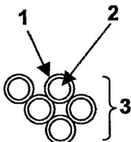
(57) Abstract: The invention relates to a filler material, especially for filling cavities, especially of structural elements, to a method of production and to a structural element. The inventive filler material comprises particles that are coated with a reactive duroplast, whereby the reactive duroplast is non-viscous at room temperature when not yet reacted.
