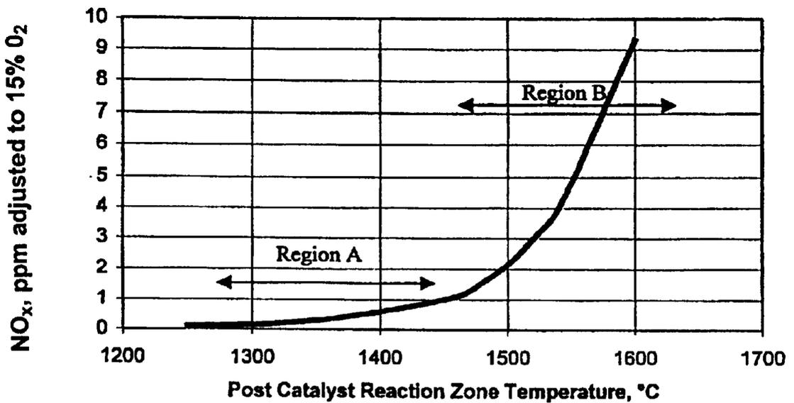
Figure 2, NO<sub>x</sub> produced vs. Temperature in a catalytic combustion system
