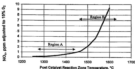
**NO<sub>x</sub> produced vs. Temperature
