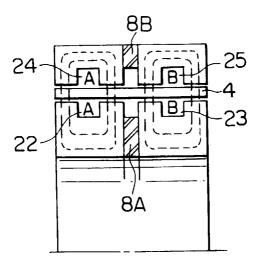
(FLOW OF MAGNETIC FLUX OF COIL)
