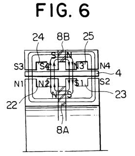
(FLOW OF MAGNETIC FLUX OF MAGNETIC PLATE)
