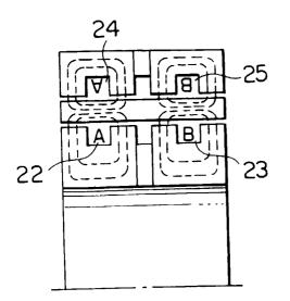
(FLOW OF MAGNETIC FLUX OF COIL)
