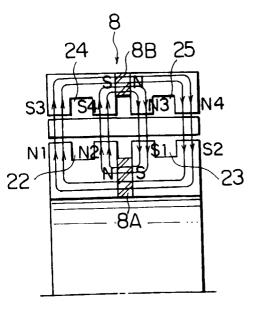
(FLOW OF MAGNETIC FLUX OF MAGNETIC PLATE)
