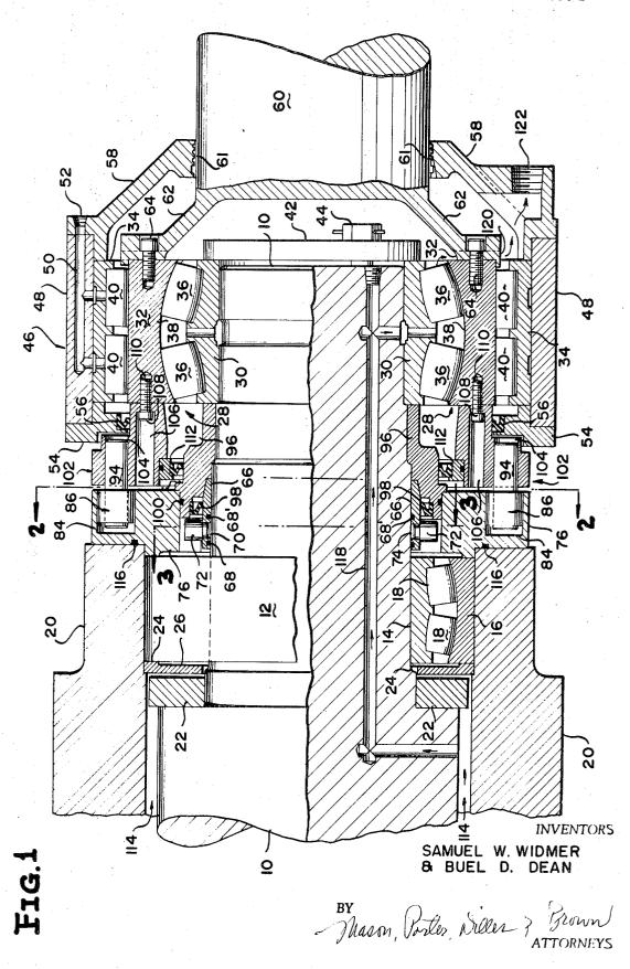
ROLL DRIVE THROUGH INTERMEDIATE RACE RING OF CONCENTRIC BEARING
