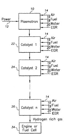
(57) Abstract: A plasmatron-catalyst system. The system generates hydrogen-rich gas and comprises a plasmatron (10) and at least one catalyst (22, 24, ..., 26) for receiving an output from the plasmatron to produce hydrogen-rich gas. In a preferred embodiment, the plasmatron receives as an imput air (14), fuel (16) and water/steam (18) for use in the reforming process. The system increases the hydrogen yield and decreases the amount of carbon monoxide.
