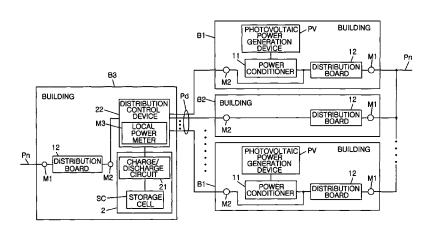
power from the common power source to the area based on the amounts of power as measured by the first power meter and the second power meter.
