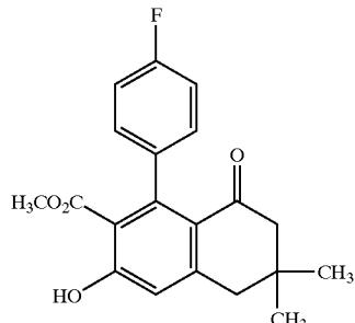
A solution of 4.0 g (11.6 mmol) of the compound of Example XIII and 13.2 g (58.1 mmol) of DDQ in 400 ml of toluene is stirred at 80° C. for 24 h. The mixture is filtered through diatomaceous earth and the diatomaceous earth is rinsed with toluene. The filtrate is concentrated under reduced pressure and the residue is chromatographed over 300 g of silica gel 60 ( $\text{CH}_2\text{Cl}_2$ ).
