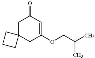
62.10 g (0.838 mol) of isobutanol and 3.4 g (0.02 mol) of p toluenesulphonic acid are added to 85 g (0.558 mol) of 5-spirocyclobutyl-cyclohexanedione in 1.8 l of toluene, and the mixture is heated with stirring on a water separator for 24 h. The mixture is cooled, washed with saturated sodium bicarbonate solution and water, dried and concentrated. This gives 121.1 g of an oil of a purity of 98.55% according to HPLC.
