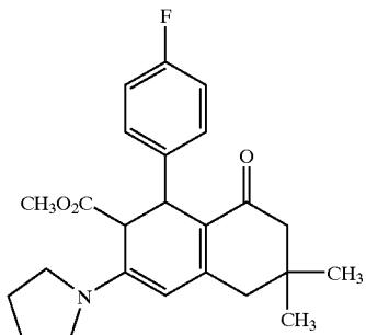
A solution of 1.69 g (10 mmol) of methyl 3-pyrrolidine-1-yl-but-2-enoate, 1.40 g (10 mmol) of dimedone and 1.24 g (10 mmol) of 4-fluorobenzaldehyde in 30 ml of cyclohexane is refluxed on a water separator overnight. The mixture is cooled, the solvent is removed under reduced pressure and the residue is purified over silica gel 60 (elution with EtOAc/toluene 1:4).
