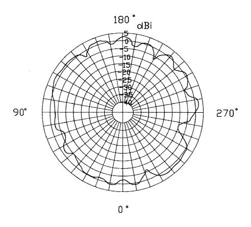
Scale: 5dBi/div Operating Frequency: 2.45 GHz Vertically polarized
