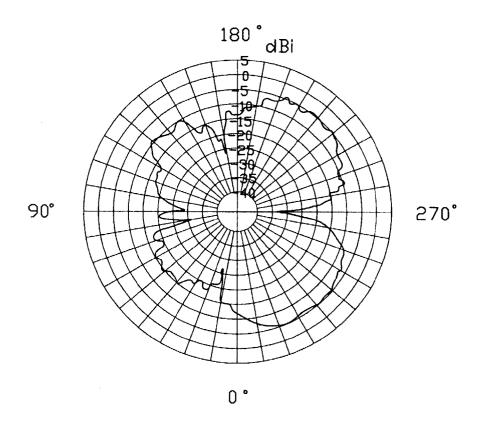
Scale: 5dBi/div Operating Frequency: 5.725 GHz Horizontally polarized
