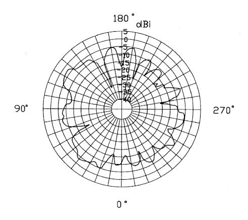
Scale: 5dBi/div Operating Frequency: 2.45 GHz Horizontally polarized
