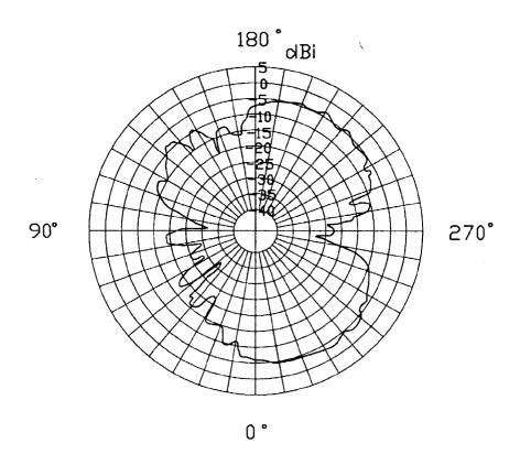
Scale: 5dBi/div Operating Frequency: 5.35 GHz Horizontally polarized
