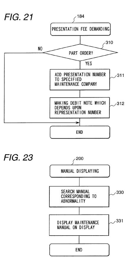
190 MAINTENANCE ORDERING ABNORMAL DATA DETECTION RECEIVE 320 MAINTENANCE <mark>ر 1</mark>91 COMPANY'S LIST DISPLAY MAINTENANCE /321 COMPANY'S LIST ON DISPLAY 322 NO IS ORDER MADE? YES MAINTENANCE ORDERING PROCESS INFORM ORDERED-323 MAINTENANCE COMPANY THROUGH MOBILE / 192 TELEPHONE DISPLAY ROOT TO 324 MAINTENANCE COMPANY BY ROOT DISPLAYING FUNCTION 194 ≻ END
