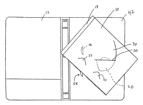
(57) Abstract: A system for mounting a component (10) to a portfolio (12) including a tongue (34) located on the component, the tongue having a tail portion and a tip portion, and a portfolio (12) having a tongue opening (50) formed therein. The top can be inserted into the tongue opening and component rotated relative to the portfolio (12) until the tongue (34) is generally received through the tongue (34) opening to couple the component to the portfolio (12).
