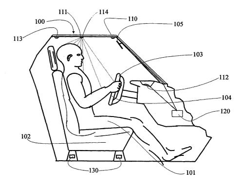
is used to affect the operation of some other system in the vehicle. When system is installed in the passenger compartment of an automotive vehicle equipped with an airbag, the system determines the position of the vehicle occupant relative to the airbag and disables deployment of the airbag if the occupant is positioned so that he/she is likely to be injured by the deployment of the airbag.
