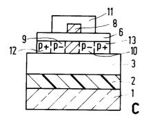
The present invention relates to a method for producing polysilicon thin film transistors (TFT) which exhibit low reverse leakage under reverse bias conditions. The instant invention further is concerned with the fabrication of low leakage, high performance polysilicon thin film transistors in which fabrication temperatures that are employed are sufficiently low so as to allow the use of commercially available glass substrates.
