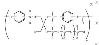
(wherein, R is alkyl group having 1 to 6 carbon atoms which may be the same as or different from each other, or a substituted or unsubstituted aromatic hydrocarbon group having 6 to 12 carbon atoms, B is  $(CH_2)_x$ , x is an integer  $_{65}$ from 2 to 6, n is an integer from 0 to 200, and m is an integer from 1 to 50), and the charge generation substance contains
