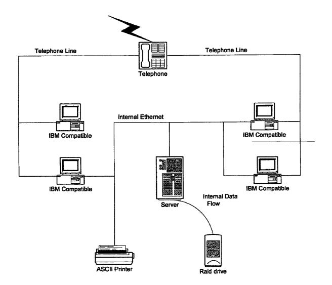
Figure 1: VariPin Assignment LAN
