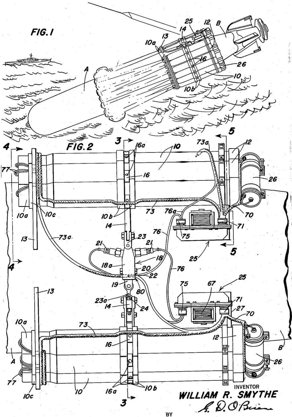
APPARATUS FOR DECELERATING TORPEDOES.
