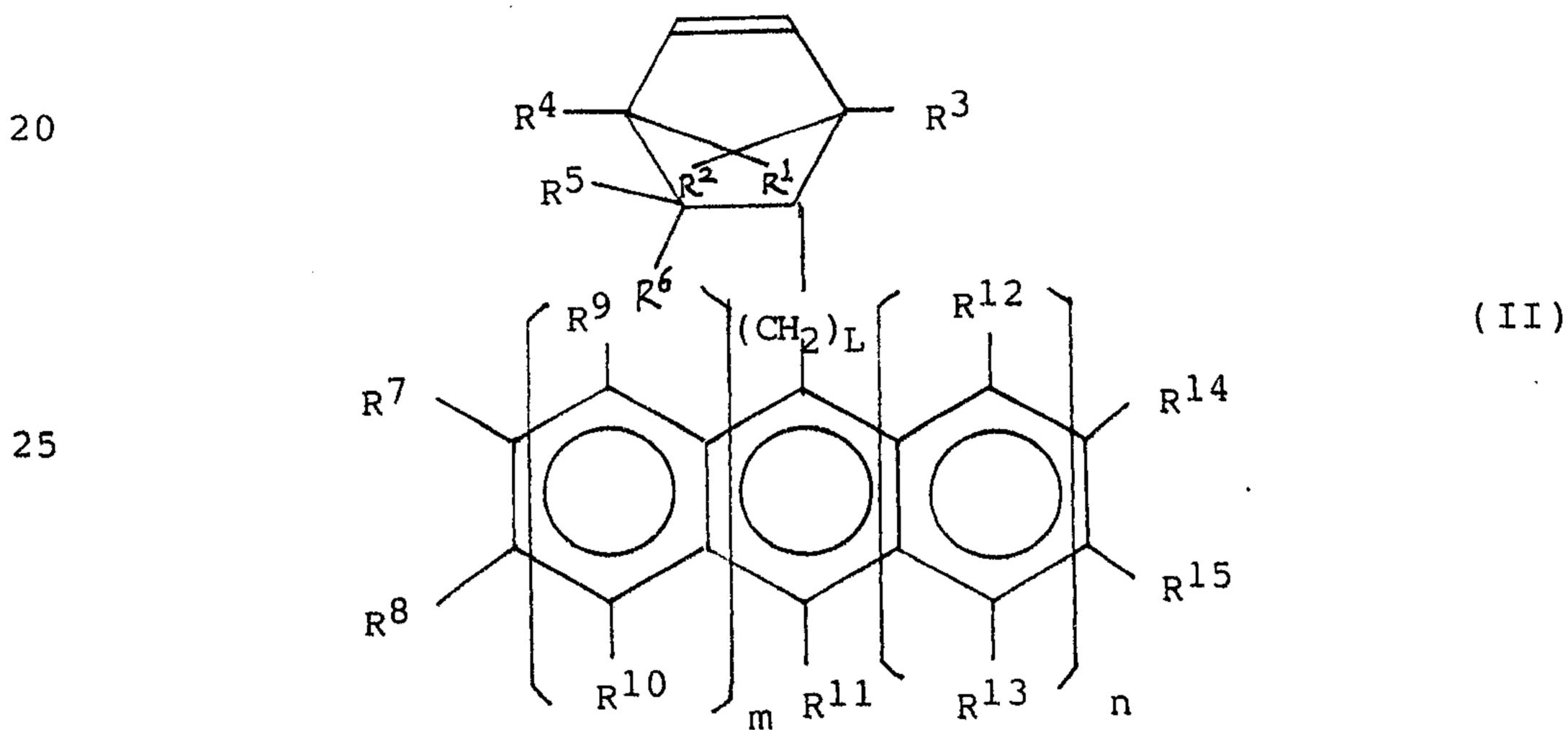
wherein L is 0 or an integer of at least 1, m and n represent 0, 1 or 2,  $R^1$  through  $R^{15}$  independently represent a hydrogen atom, a halogen atom, an aliphatic hydrocarbon group, an aromatic hydrocarbon group or an alkoxy group, and  $R^5$  (or  $R^6$ ) and  $R^9$  (or  $R^7$ ) may be bonded together through
