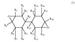
(where, R<sub>1</sub>-R<sub>18</sub>, which may be same or different, comprise either hydrocarbon groups that may contain a hydrogen atom, a halogen atom, an oxygen atom, or alkoxyl groups that may contain a substitution group).
