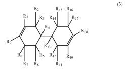
(where,  $R_1$ - $R_{18}$ , which may be same or different, comprise either hydrocarbon groups that may contain a hydrogen atom, a halogen atom, an oxygen atom, or alkoxyl groups that may contain a substitution group).
