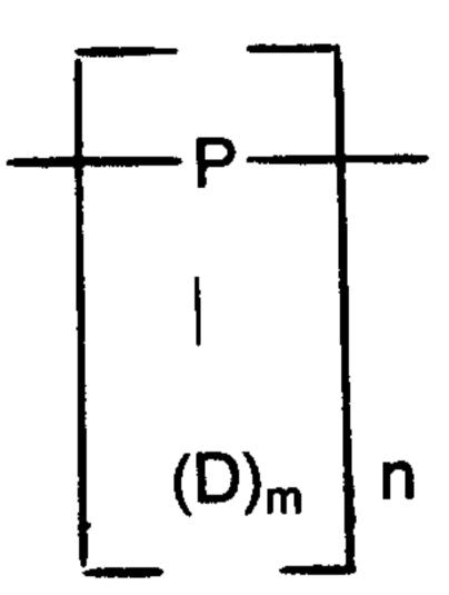
wherein m is from 0 to 2; n is selected to provide a molecular weight of from about 500 to about 1,000,000; each P and each D can contain one or more moieties selected from the group consisting of =N-C(=0)-, ≡N → 0, and mixtures thereof, such that said structure provides dye transfer inhibition and has a water solubility of at least 100 ppm.
