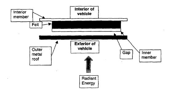
FIG. 3 **Summer Conditions** Temperature measured between interior member and felt
