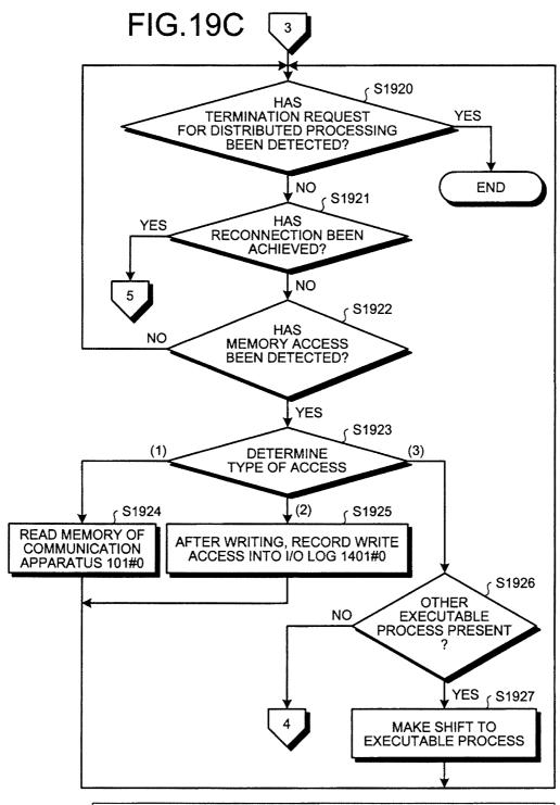
(1): READ ACCESS FOR DATA SPECIFIC TO PROCESS ON COMMUNICATION APPARATUS 101#0 (2): WRITE ACCESS FOR DATA SPECIFIC TO PROCESS ON COMMUNICATION APPARATUS 101#0
