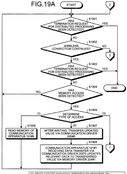
(1): READ ACCESS FOR DATA SPECIFIC TO PROCESS ON COMMUNICATION APPARATUS 101#0
