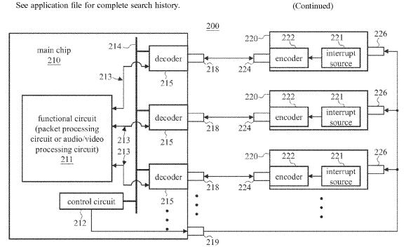
decode the digital data to obtain the data segments and the interrupt message. The control circuit is coupled to the decoder and is configured to process the interrupt message.
