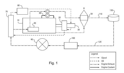
(57) Abstract: A fluid heating process which does not utilize an open flame, heat is created by a rotating prime mover(s) driving a hydraulic heat generator. Heat is also collected from the prime mover cooling system, and any exhaust heat generated by the prime mover. The heat energy is collected from all these sources, and transmitted through heat exchangers to generate a hot fluid, which can be used to heat other fluids and used for any application where heat is required.
