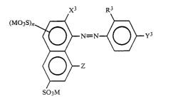
where n is an integer of 0 or 1,  $X^3$  represents hydrogen or  $--NH_2$ ,  $Y^3$  represents hydrogen or  $--NHR^1$ wherein R<sup>1</sup> represents an alkyl group, Z represents hydrogen, -OH or -COOM, and R<sup>3</sup> represents hydrogen, an alkyl group or  $-SO_3M$  wherein M is the same as that defined in formula III;
