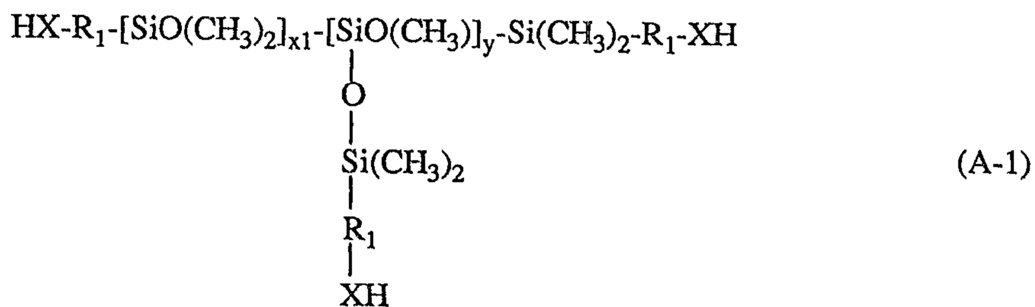
wherein X is oxygen, sulfur, -NH- or -COO- (which is bound with its carbon atom to R<sub>1</sub>), R<sub>1</sub> is a linear or branched alkylene group with 2-7 carbon atoms, x<sub>1</sub> is an integer from 10-100 and y is 0 to 4;
