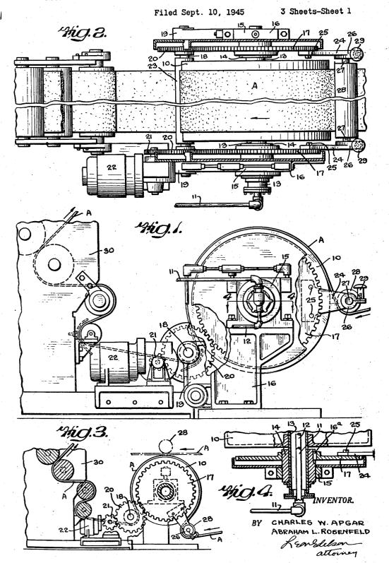
ROTARY DRUM DRYING APPARATUS HAVING MEANS TO GUIDE WEB OVER DRUM
