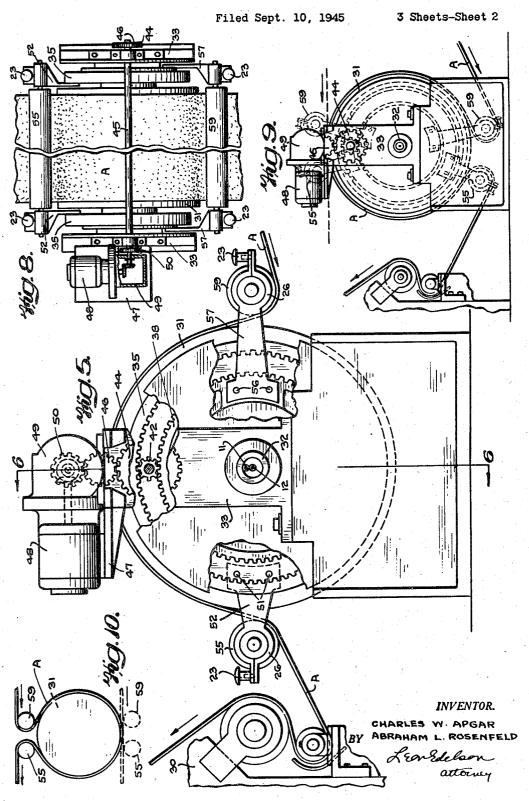
ROTARY DRUM DRYING APPARATUS HAVING MEANS TO GUIDE WEB OVER DRUM
