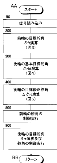
FIG. 2: 50 Read signals 200 Calculate target steering angle \delta_{rt} for front wheels (fig. 3) 300 Calculate basic target steering angle \delta_{rbt} for rear wheels (fig. 4) 400 Calculate target corrective steering angle \Delta\delta_{rt} for rear wheels (fig. 5) 800 Implement front wheel steering angle control 900 Implement calculation of target steering angle \delta_{rt} for rear wheels and steering angle control AA Start BB Return
