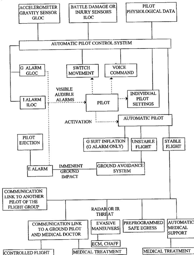
FIGURE 1 Automatic pilot control system for GLOC or ILOC with a pilot ejection system and medical support, and a communications link to another pilot, a ground pilot, or medical doctor.
