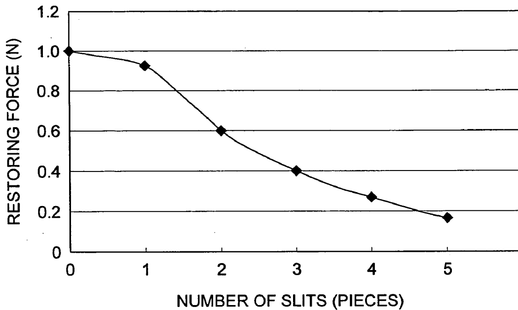
RELATIONSHIP BETWEEN NUMBER OF SLITS AND RESTORING FORCE (AMOUNT OF DISPLACEMENT 1 mm)
