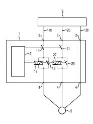
step, the switch element first closes and then switches the semiconductor switch to be conductive.
