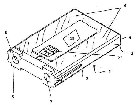
(57) Abstract: A fluid separation conduit cartridge comprising a fluid separation conduit is disclosed. In certain embodiments the fluid separation conduit is potted to provide operation at increased pressures. In other embodiments, the fluid separation conduit cartridge has one or more memory units. The memory units are operative to store data such as, for example, cartridge usage and test results
