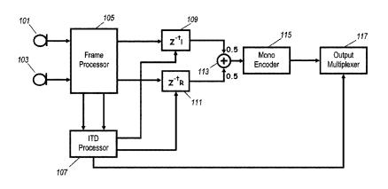
difference may specifically be determined by an algorithm based on determining cross correlations between the first and second audio signals.
