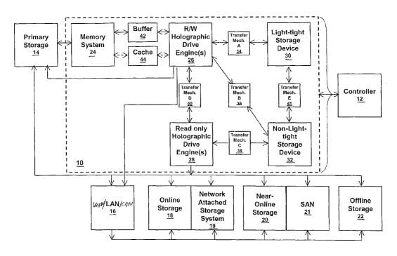
(57) **Abstract:** A hybrid data storage system that includes a controller that communicates with an outside source of information, and at least one holographic drive engine that communicates with controller. The information is transmitted between the controller and the outside source of information and between the holographic drive engine and the controller.
