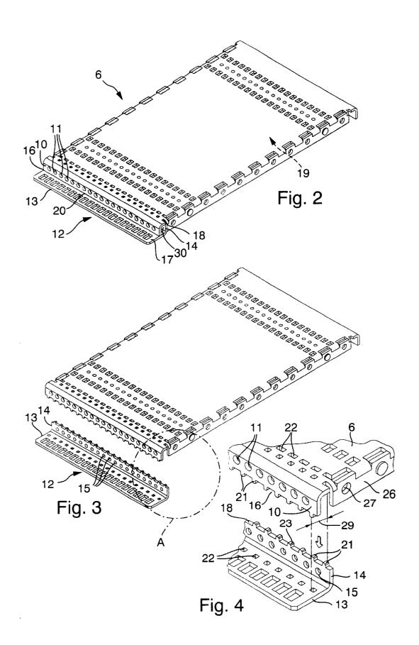
the case may be. The bent section exhibits a series of holes that are aligned with the threaded holes, and along the longitudinal edge of the bent section and the outer edge provision is made for connecting means.
