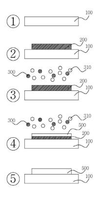
Cyclotron Resonance Plasma Enhanced Chemical Vapor Deposition; ECR-CVD)을 수행하되,
